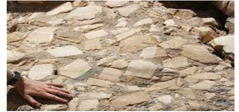
Name this Sedimentary Rock. Clastic Fragmental texture, composed of cobble, pebbles and boulder, embedded in clay or sand, Mostly Quartz and Feldspar, Angular Fragments
